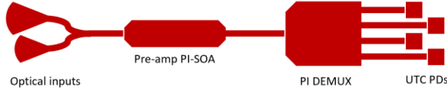
Figure 8.1: Simplified architecture of the optical part of the receiver
