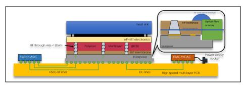
active and passive components co-integrated on the same chip to enable all necessary transceiver functionalities.
