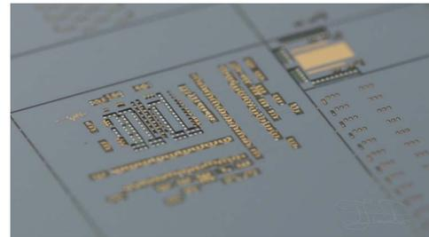
Fig. 5. Picture of a part of the co-integrated wafers, showing InP membrane layer with windows opened to access and interconnect the contact pads of photonics (gold) and electronics (aluminum) [15].
