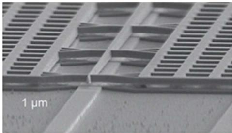
Fig. 3. Picture of the double-waveguide NEOMS on IMOS [11].
